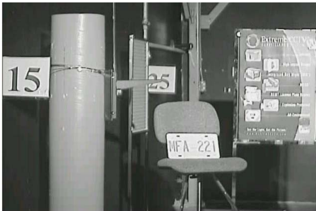
Trial 4: infrared on. Bit rate = 1.21 mbps. Bit rate reduction = 91%.
